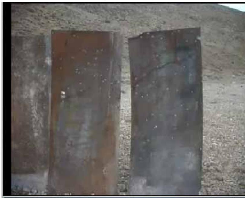
Damage shown from shrapnel after the test.
