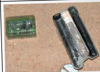
IR Transmitter (Left) with Ultraviolet Ink (Right) for Marking Targets
